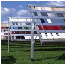
One year of testing in South Florida at 45° S. is equivalent to two years on a roof and three years on a wall north of Jacksonville, FL.
