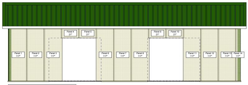
Shift the vertical starting point of the first panel to 1 1/2 in. from the outside corner of the building so there is no panel rib & steel corner trim conflict at the other end. The rib spacing will also be balanced.
